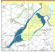
Under a 2m sea level rise scenario the most significant change in flood risk would be at the head of the Dulas estuary and along the valley of the Afon Goch. The adjacent plot shows a comparison of the projected MHWS levels under the 1m and 2m sea level rise scenario. Under the 2m scenario there could be normal tidal inundation of some properties and the road at City Dulas would be affected.
