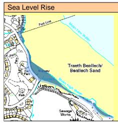
Under a 2m sea level rise scenario there is the possibility of direct flooding under normal tidal levels to the properties at the north end of the Benllech frontage. The adjacent plot shows a comparison of MHWS flood extent for MHWS under the 1m and 2m water level scenarios. Under a 2m scenario the southern end of the road would be submerged on MHWS, highlighting not only this future risk but also the vulnerability of this corner to direct flooding and wave overtopping at present.
