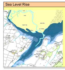
The adjacent plot shows a comparison between projected MHWS for the present day, the 1m scenario and 2m scenario. Under the 1m scenario the effective entrance would increase in width and under a 2m scenario there would be significantly greater flooding over much of the western frontage.
