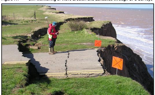
Figure 7.1 Cliff Monitoring of Wave Erosion and Landslide through GPS Surveys
